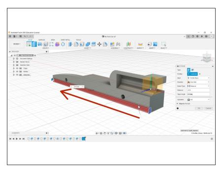
Extrude cut the rectangle to a distance of -210mm (All of the way through the car).
