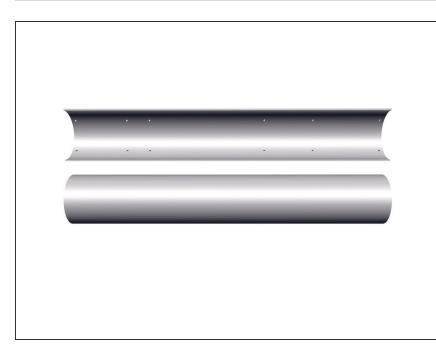
• 2 x 690mm PVC Pipe Halves are required for the Hull Assembly
