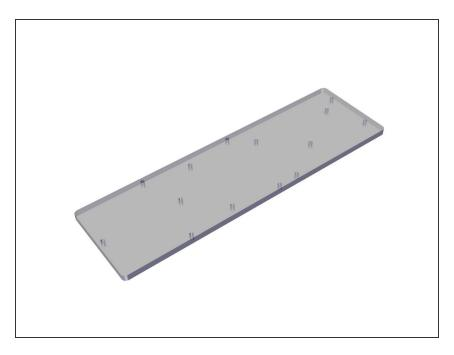
• 1 x Laser Cut PPM Support Plate is required for the PPM Assembly
