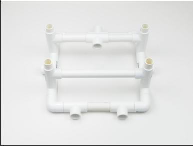
Insert 4 of the 32mm Connectors into the upright Tee Joints of the frame.
