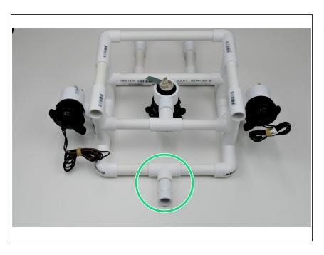
Mount the Tether Input into the rear Tee Joint of the ROV.
