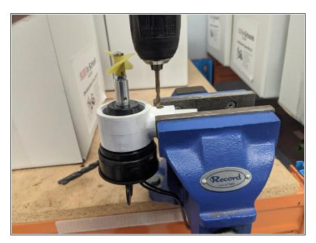
Mount the motor assembly in a vice, ensuring the surface to be drilled is held at a 90\* angle.
