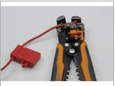
Using your wire strippers, strip 15mm from the ends of the red fuse wire and the red power wire.
