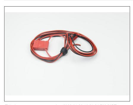
Cut the two terminal ring connectors from the end of the power wires.
